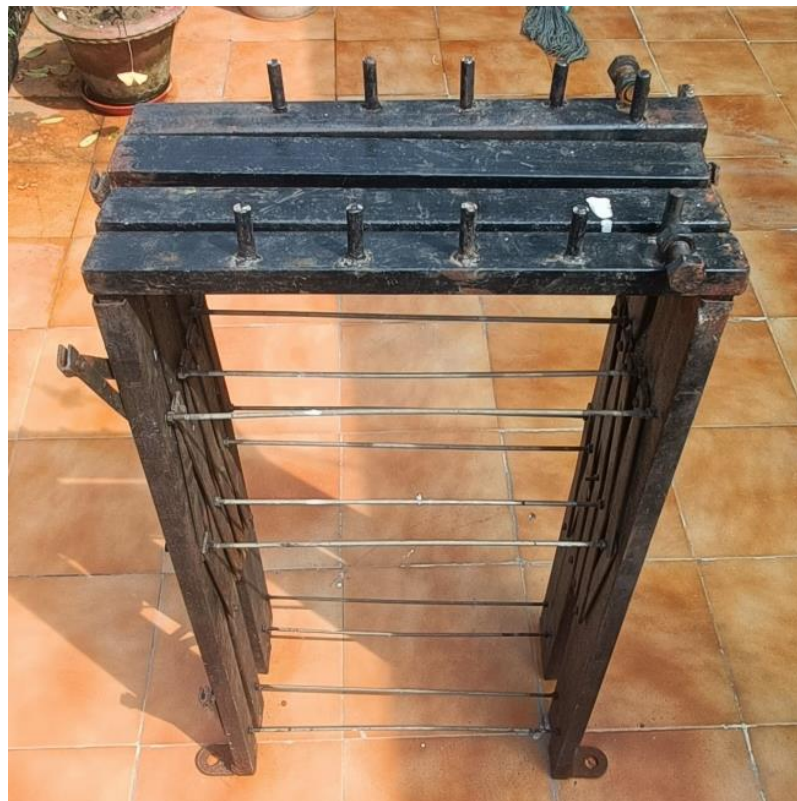
(d) Fabricated Foldable multitasking workable platform (Arrangement for making stirrups)
