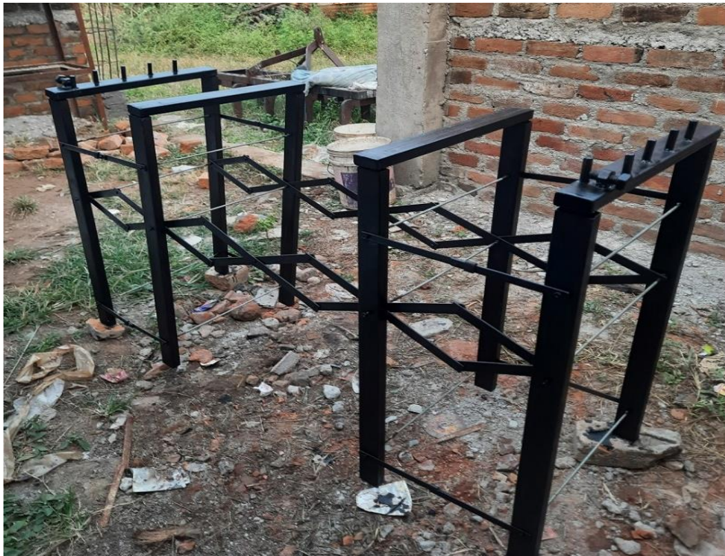
(a) Fabricated Foldable multitasking workable platform
