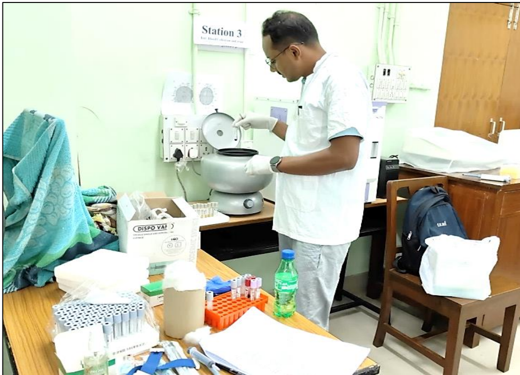
Figure 17: Centrifugation (Serum Separation): 5-10 minutes at 1,000-1,500 x g 3 .
