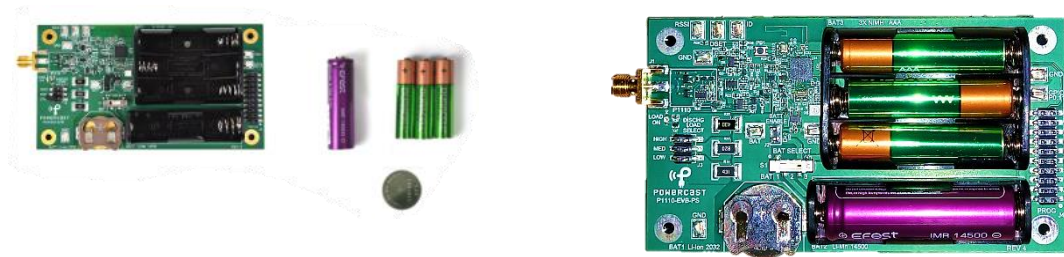
Fig 7.3 Powerspot Development Board with battery holder for harvesting energy to charge the on-board batteries [11]
