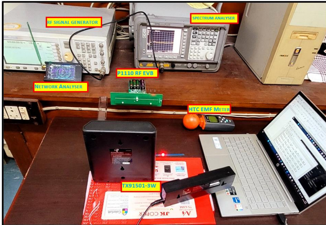
Fig. 7.5 Experiment Setting for monitoring Battery Recharge Time at 915 MHz
