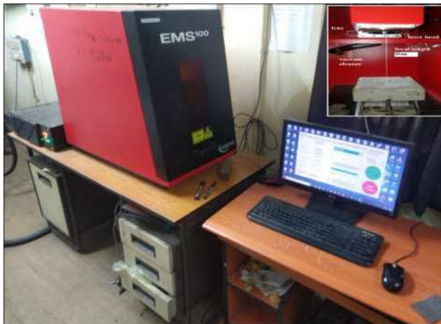
Figure 2.4. Laser welding setup
