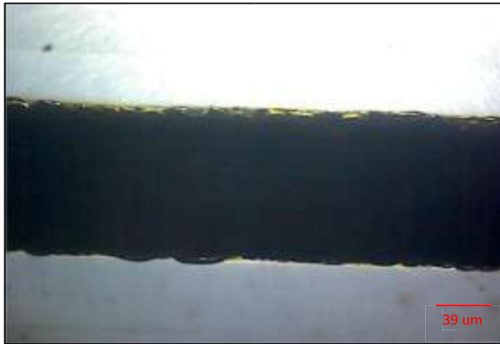
Figure 3.4. Microscopic image of sample having minimum HAZ (20.85 \mu\text{m} )
