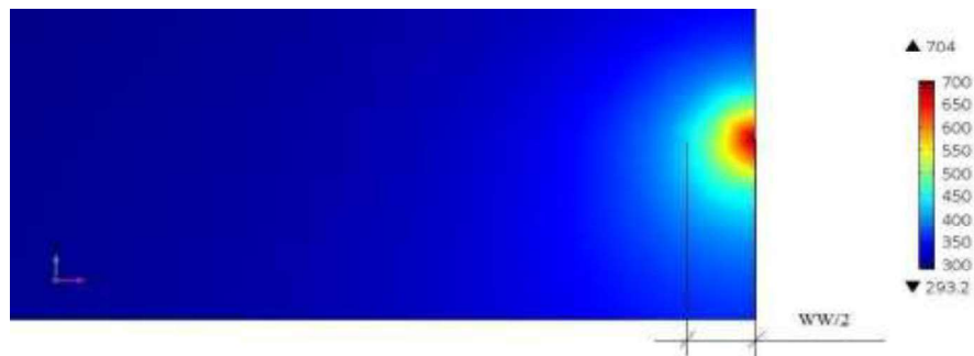
Figure 3.14. Temperature contour of the interface for weld width measurement
