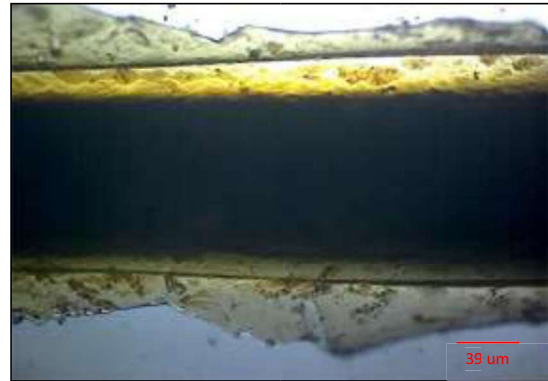
Figure 3.5. Microscopic image of sample maximum value of HAZ (105.8 \mu\text{m} )
