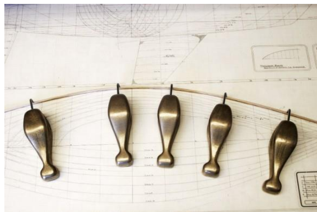
Figure 3.8: Hooked weights, called “ducks,” accurately secure a spline – here, no more than a thin strip of balsa – for tracing the hull of a sailing vessel. Source: Edson International [109]
