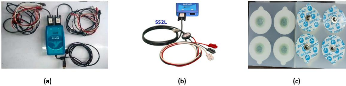
Fig. 3.1 (a) Biopac MP45- Two-channel data gathering device, (b) Biopac electrode Lead set (SS2L), (c) Biopac disposable electrodes (EL503).
