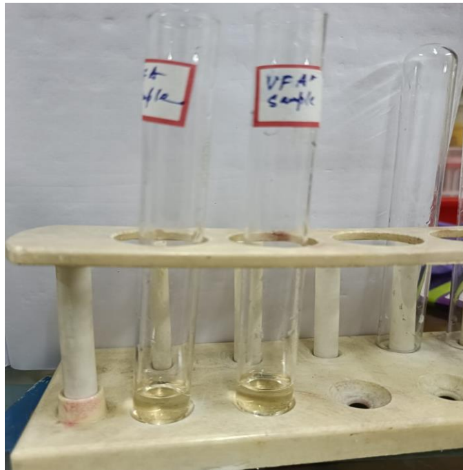
Figure 18: Color development after the addition of \text{FeCl}_3
