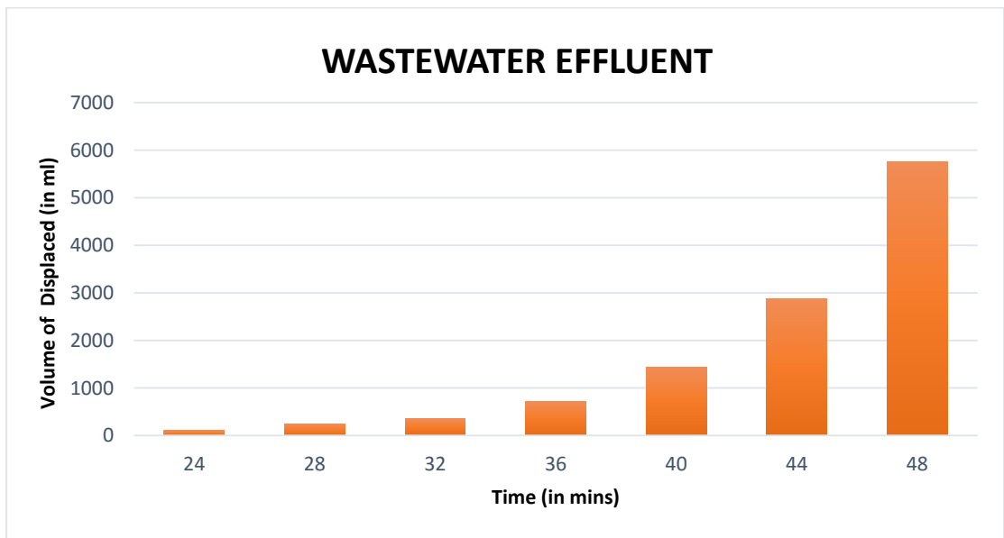
Figure 32: Displacement of gas using Wastewater effluent
