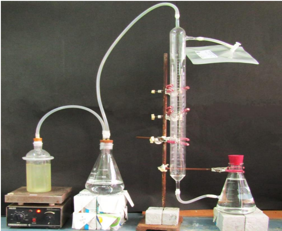
Figure 25: Experimental setup for bio-hydrogen production
