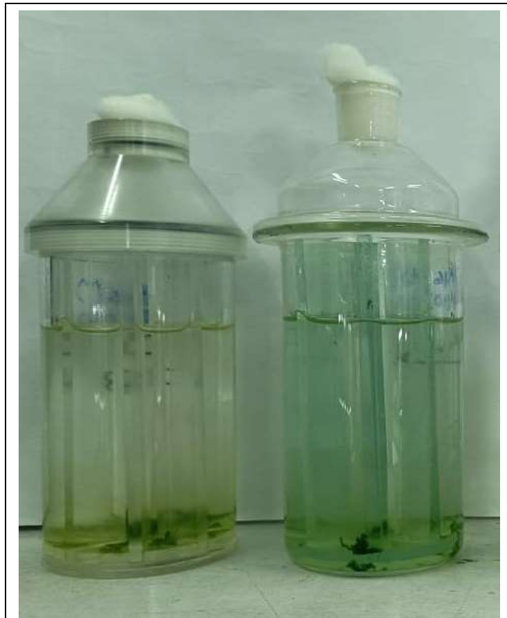
Figure 3: Biofilm culture in two conico cylindrical flasks (CCF) made of PMMA and glass.
