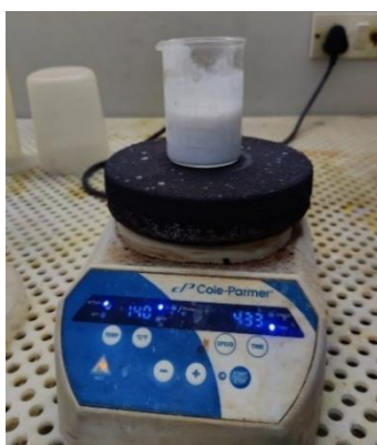
Fig. 4.11 Magnetic stirring process on a Hot-Plate.
