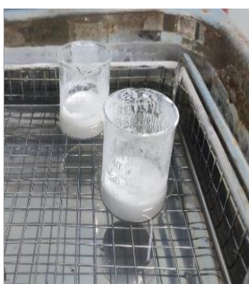
Fig. 4.10 Ultrasonification Process in Ultrasonic Cleaner
