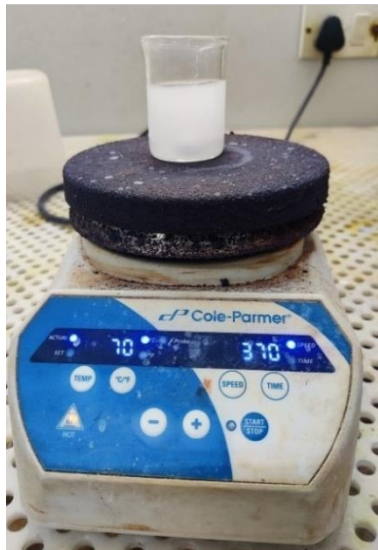
Fig. 4.20 Magnetic Stirring Process of the solution.
