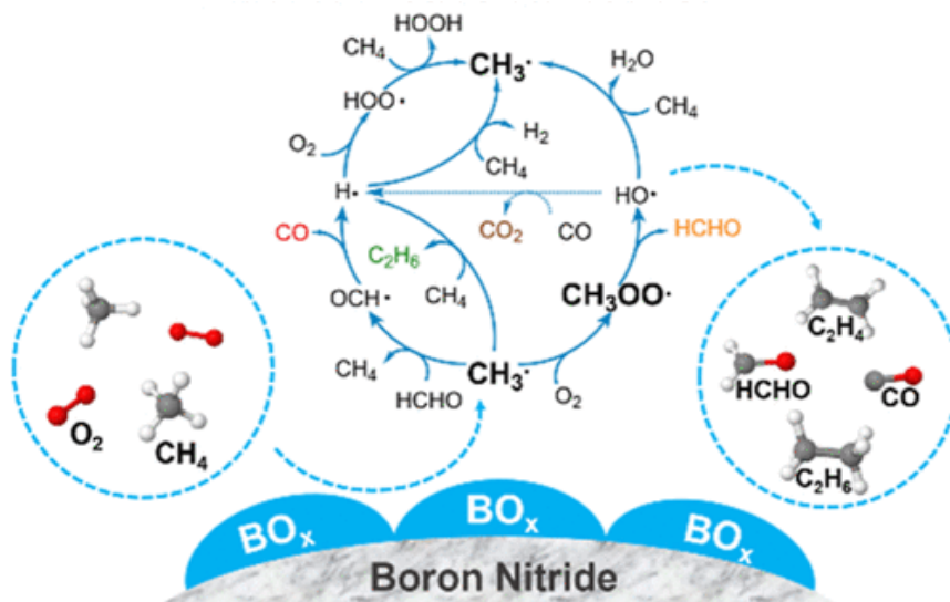
Fig. 3.28 Ion absorption Model: Boron Nitride reaction with Methane molecule. [113]
