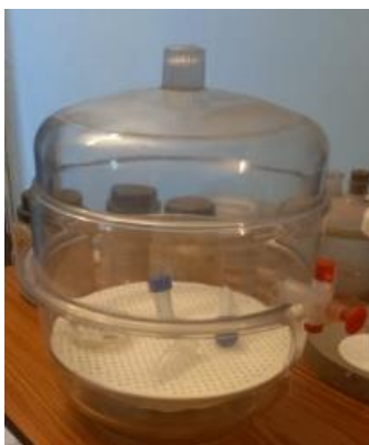
Fig. 4.12 The Precipitate being vacuum dried in a Desiccator.
