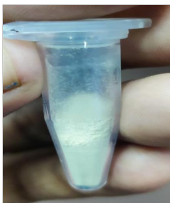
Fig. 4.13 The resulting BN QDots (powder form) stored in a centrifuge tube.
