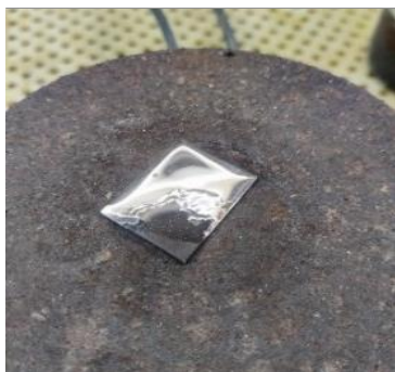
Fig. 4.16 The sample is heated to settle down the nanoparticles.
