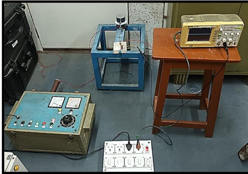
Figure.4.13: Actual diagram of the LC measurement setup
