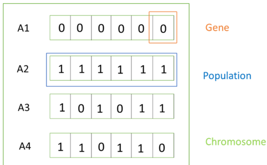
Figure 3.2: Feature Selection using Genetic algorithm
