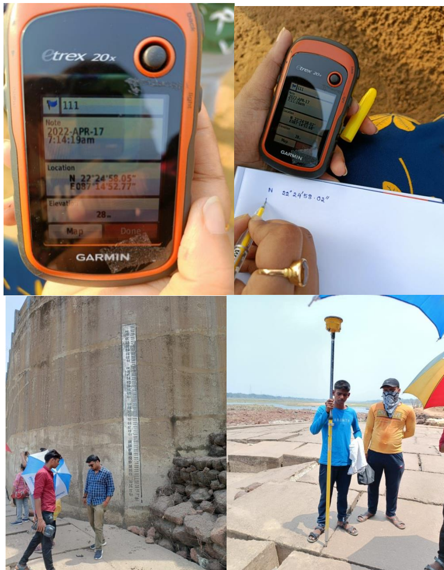
Fig: 4.2 Measuring latitude/longitude and elevation by GPS
