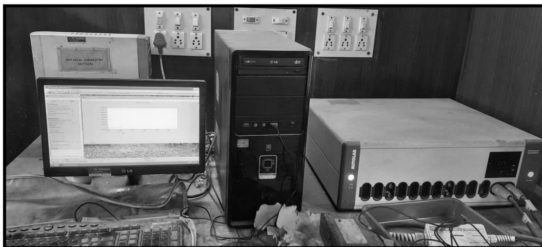
Figure I.5 Potentiostat for electrochemical measurement
