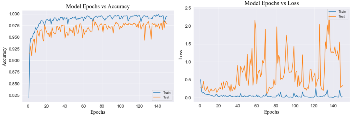
Figure 4.4: (a) Accuracy Plots for Training and Testing (b) Loss Plots for Training and Testing obtained using feature extractor model for UCI-HAR dataset
