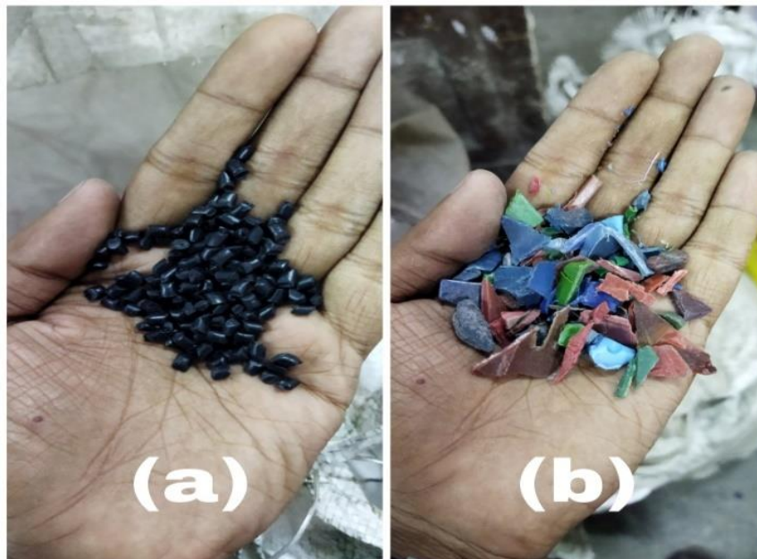
Figure 4.1: (a) PE based fine aggregate; (b) PET based coarse aggregate
