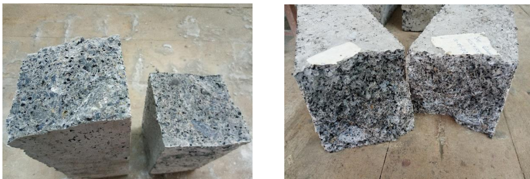
Fig. 4.11 Failure surface of flexural strength test specimens after testing
