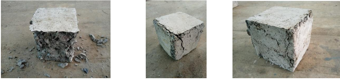
Fig. 4.15 Study of temperature test specimens of M25 grade mixes with 5%, 10% and 15% rubber content
