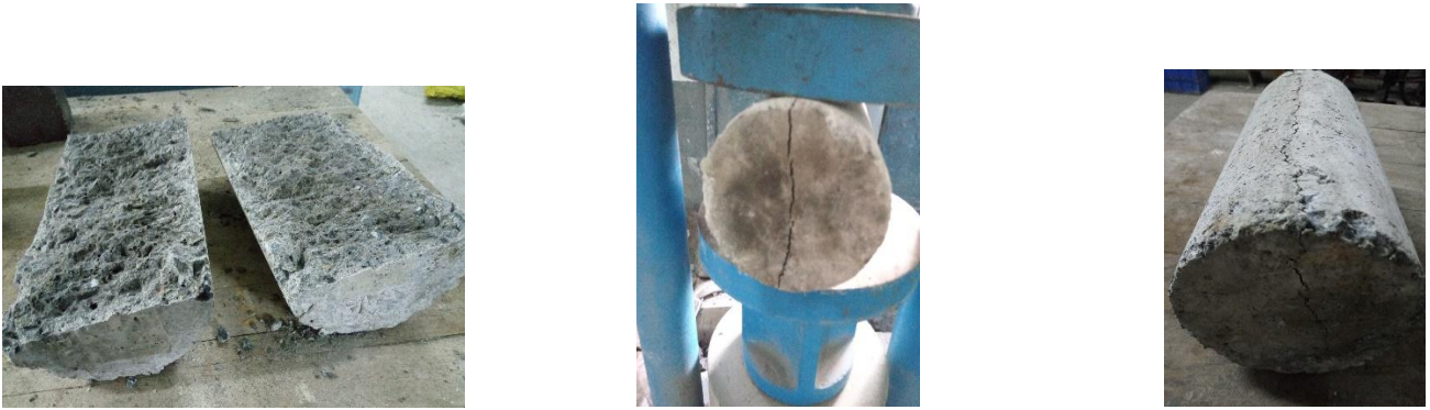
Fig. 4.9 Split tensile strength test specimens of M25 grade mixes with different rubber content
