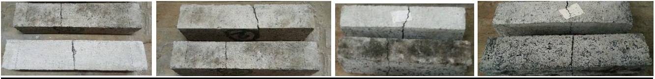
Fig. 4.12 Flexural strength test specimens of M25 grade mixes with different rubber content
