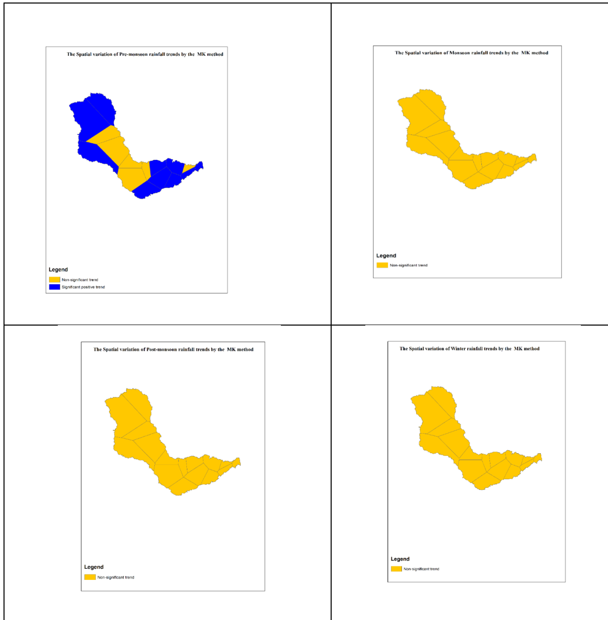
Fig 5.8(b) Spatial distribution of Pre-monsoon, Monsoon, Post-monsoon and Winter rainfall trend identified by MK test at 5%,10% significance level.
