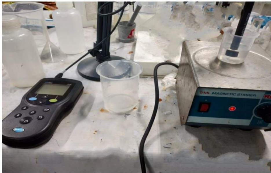
Fig. 8: Ion Selective Electrode Method
