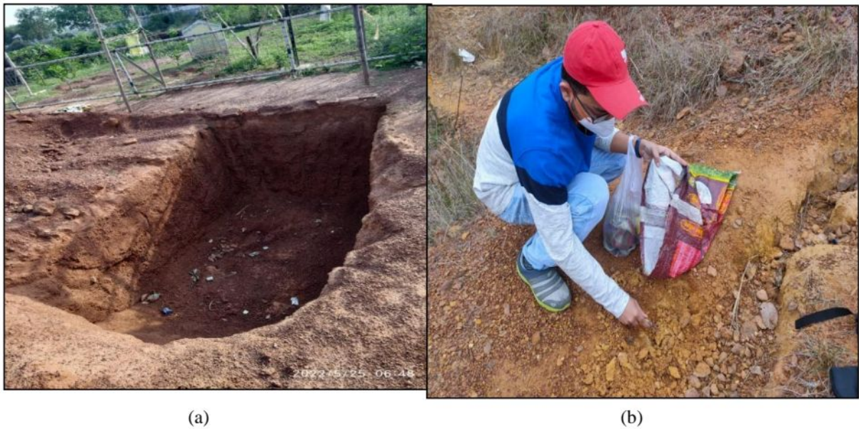
Fig. 5: Laterite Soil sample collection (a) Red Laterite (b) White Laterite
