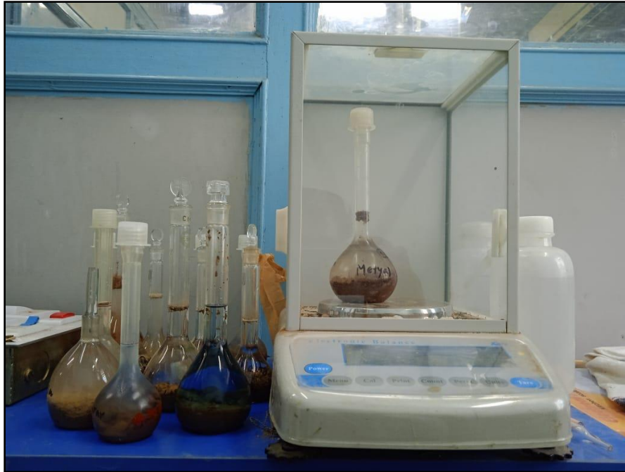
Figure 26 Specific gravity test arrangement in laboratory
