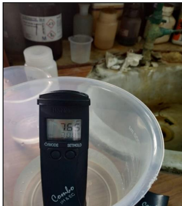
Figure 5 Probe to measure pH, TDS & EC
