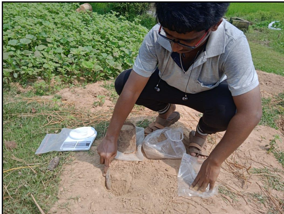
Figure 27 Field level bulk density determination using core-cutter
