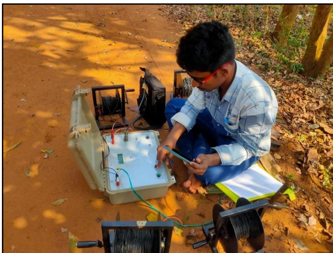
Figure 4 Vertical Electrical Sounding survey in the field
