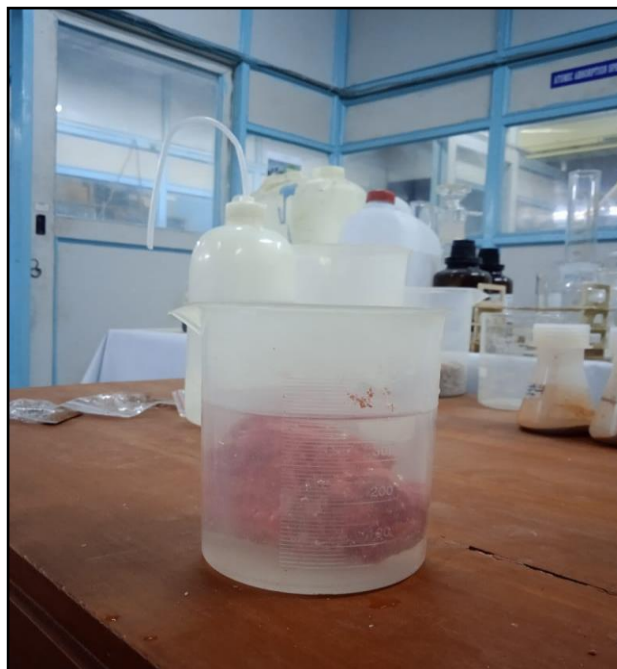
Figure 28 Determination of bulk density by water displacement method
