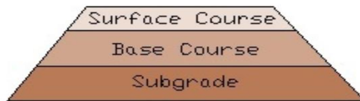
Figure 1.1: Typical cross-section of a rigid pavement [8]
