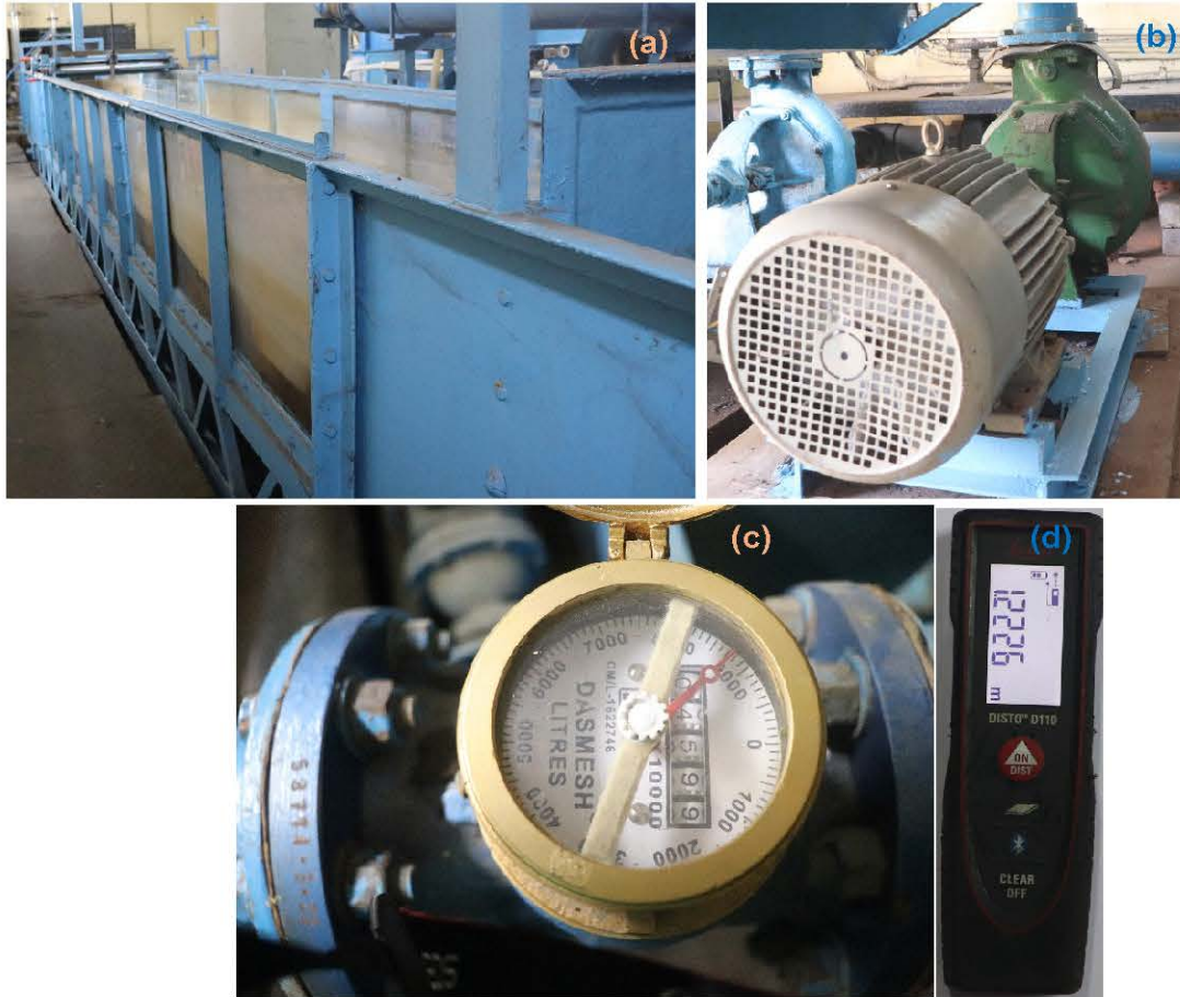
Fig. 8.1 Shows (a) tilting flume, (b) centrifugal pump, (c) flowmeter, and (d) laser distance meter.
