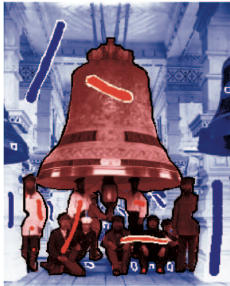
Figure 2.3: Segmentation of the people and bell in the foreground from the background area using graph cut with seeding [6]
