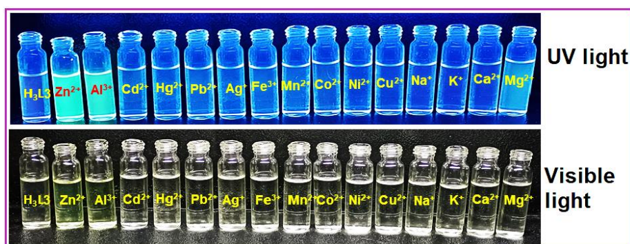
Fig. 3.17. Colour changes of chemosensor ( H_3L3 ) (20 \mu M) under UV and Visible light when different metal ions in HEPES buffer (1:9, MeOH:H 2 O, v/v, pH 7.4) medium are present.
