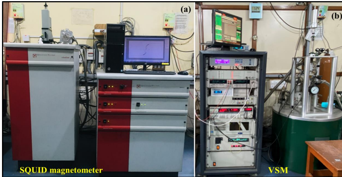
Figure 2.15: (a) The Superconducting Quantum Interference Device (SQUID) and (b) Vibrating Sample Magnetometry (VSM)
