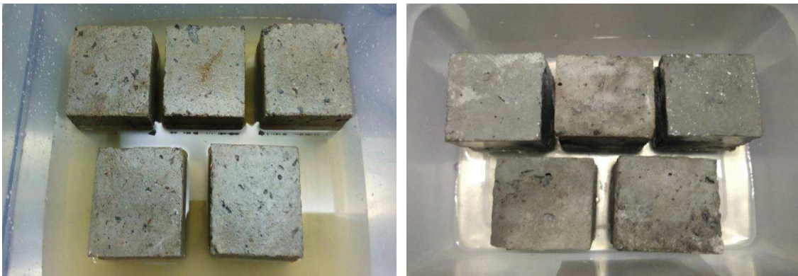
Fig. 2 Experimental set up for deterioration test of: a) M40 grade concrete (10 cm x 10 cm x 10 cm); b) M20 grade concrete (5 cm x 5 cm x 5 cm) cubes.
