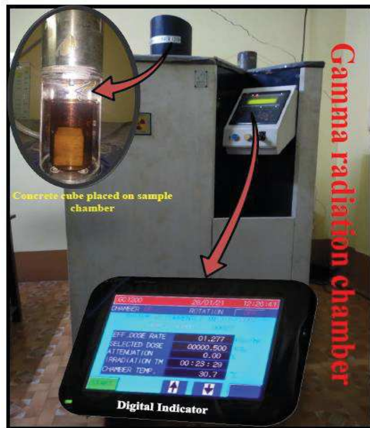
Fig. 4.8 Concrete cubes were irradiated with selected dose in gamma radiation chamber.
