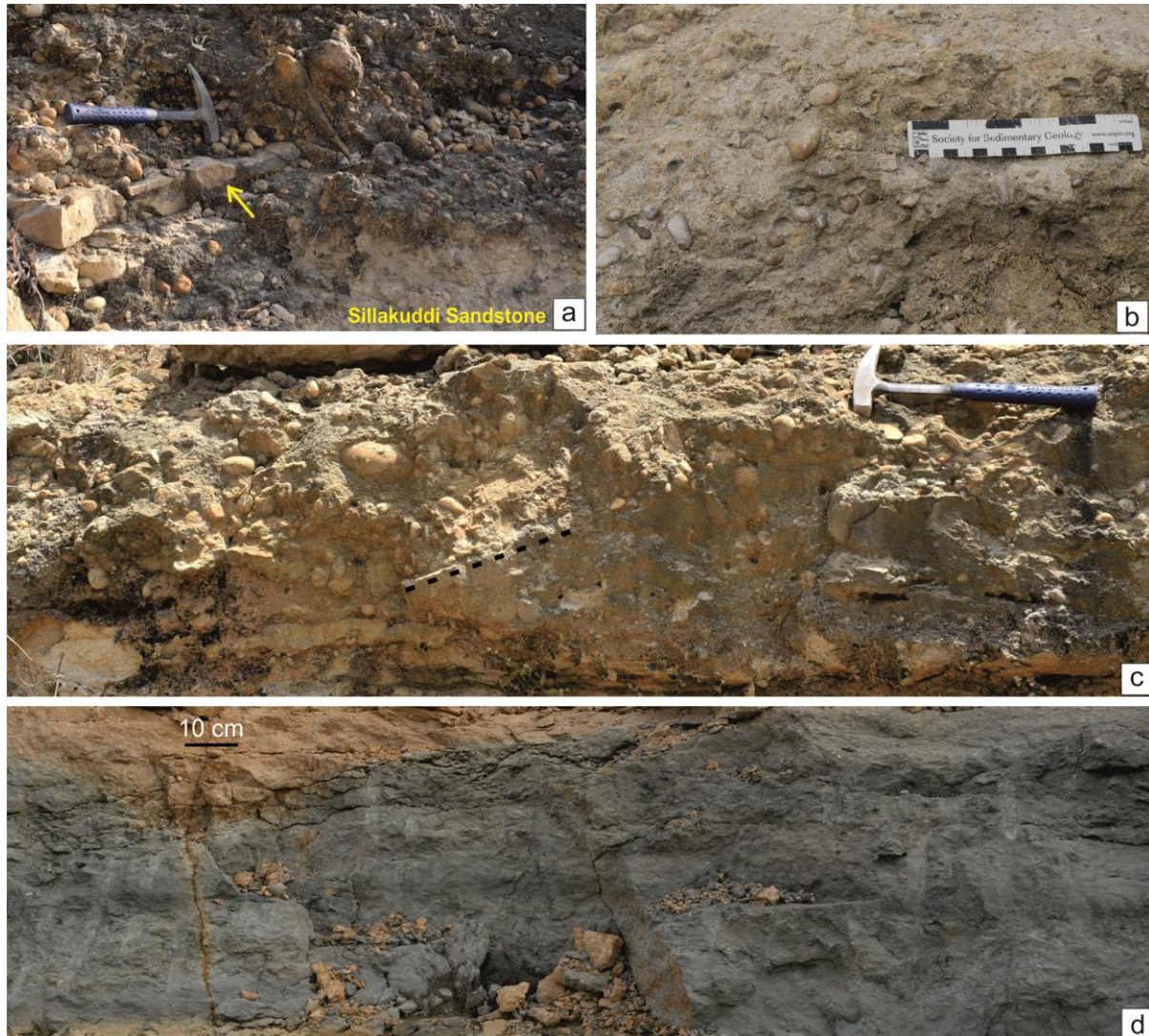
Fig. 7.2 Clast-supported scree conglomerate present at the basal part of the Kallankurichchi Formation. Note, the maximum length of clast (arrowed yellow) (a); matrix-supported conglomerate overlying scree conglomerate (b); syn-sedimentary slide planes present within conglomerate (dotted) (c); dark-grey limestone overlain by the yellowish fossiliferous limestone (d). Note Hammer length = 30 cm.
