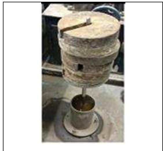
d) Soil slurry loaded for consolidation
