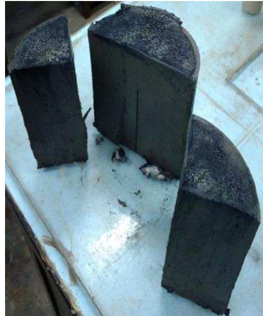
b. Using wire and knives the consolidated sample being shaped for triaxial testing
