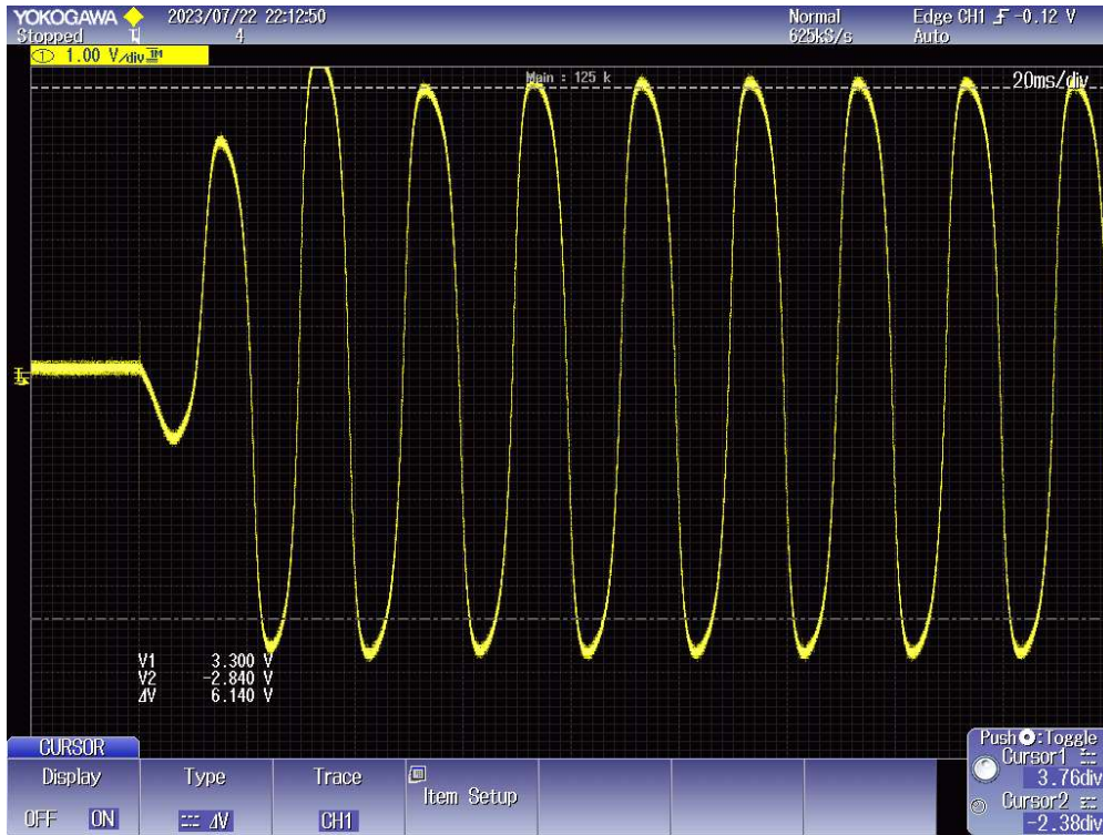
Fig. 3.17. Capacitor voltage at 210 V supply voltage
