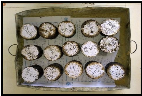
Figure 5.5 Marshall Test sample
