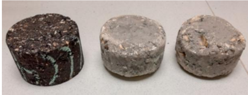
Figure 6.13 Cantabro Abrasion Unaged & aged samples
