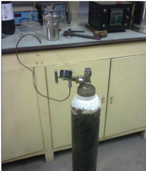
Fig. 3.19 Oxygen Cylinder to maintain pressure of 30\text{kg/cm}^2
