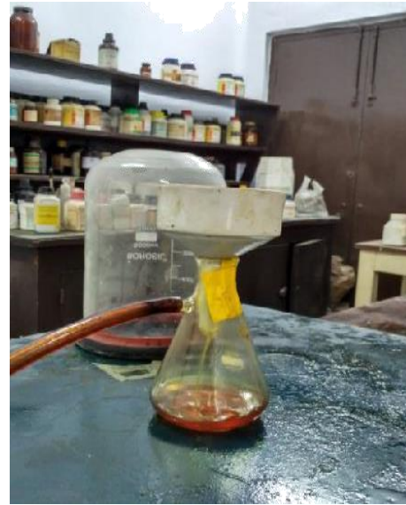
Fig. 3.5 Filtered oil obtained by vacuum filtration
