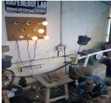
Fig. 6.2 Test engine setup run by biodiesel blends and diesel
