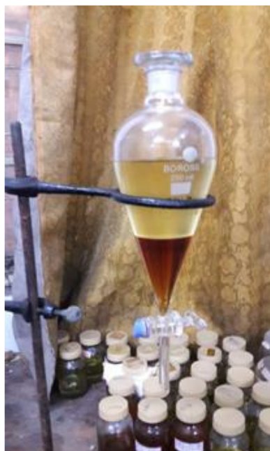
Fig. 3.10 Separation of biodiesel and glycerine
