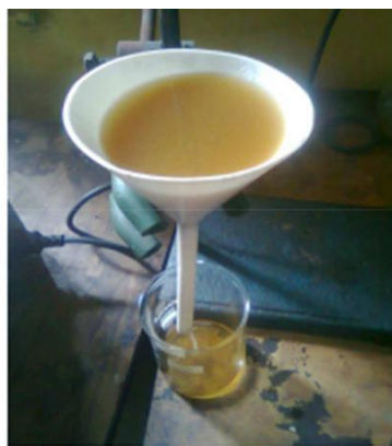
Fig. 3.3 Gravity Filtration through cotton wool
