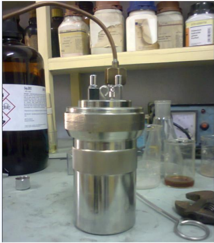
Fig 3.17 Bomb or vessel in which combustion takes place
