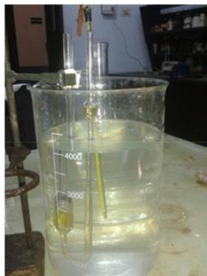
Fig. 3.15 Viscosity measurement using Ostwald's Viscometer
