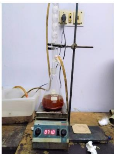
Fig. 3.7 Transesterification set up with heating and stirring
