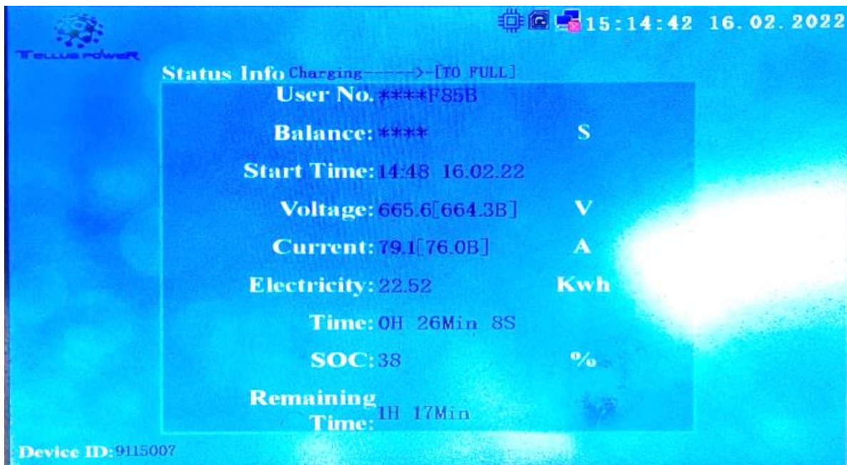
Fig. 2.8: Screen of DC slow charger while charging 2
