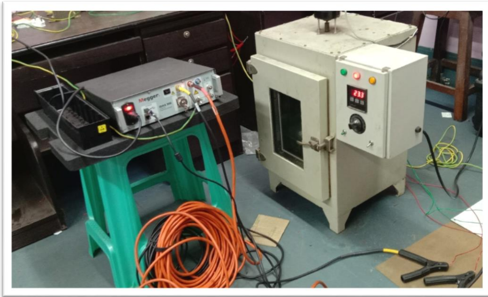
Fig. 4.12. IDAX and nano sample connection.
