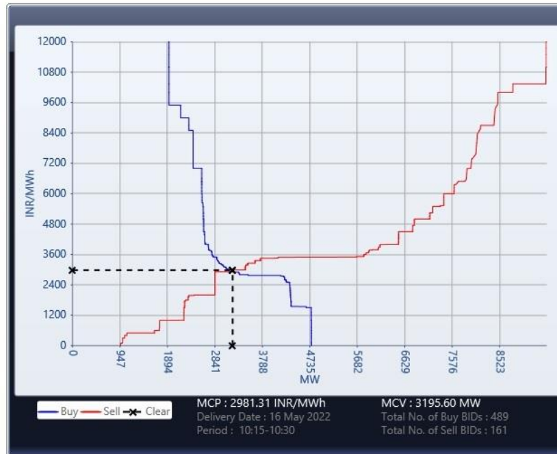
Fig 2.10 Aggregated Demand Supply plot of a 15 min (10:15 – 10:30) time block of 16 th May, 2022 (Day ahead market)
