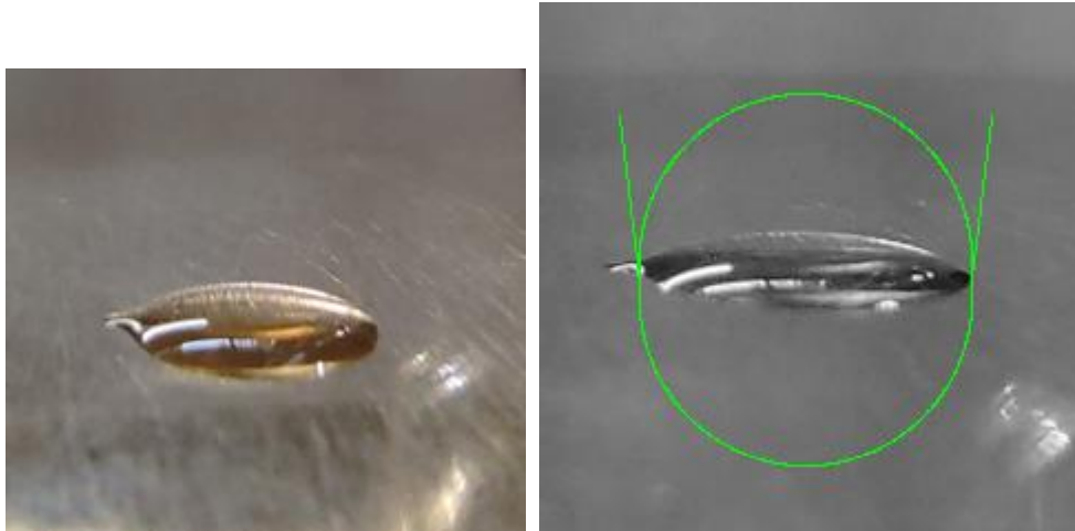
Fig.4.32 Propanol2 droplet from burette dropper on brass substrate and its contact angle drop analysis image J software.
