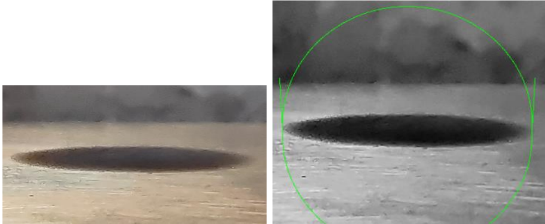
Fig.4.46 CuO-Propanol2 droplet on brass substrate and its contact angle drop analysis by image J software.
