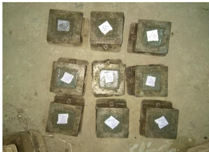
Fig 3.14: Specimen preparation for compressive strength test.
