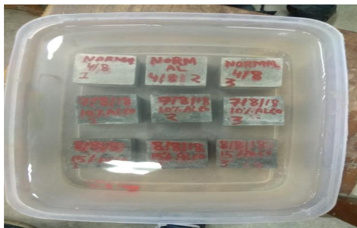
Fig 4.78 Sample Exposed to 4% MgSO_4 Solution.
