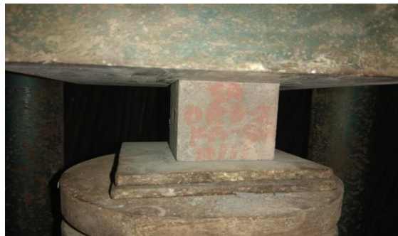
Fig 4.55 Compressive strength test setup.
