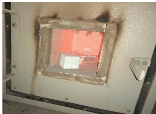
Fig 4.89 Sample exposed to elevated temperature up to 800°C
