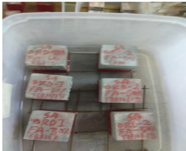
Fig 3.16 Sorptivity test setup
