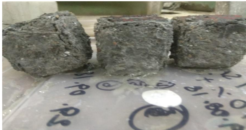
Fig 4.67 Physical condition of the Samples after 56 days Sulphuric acid exposure.
