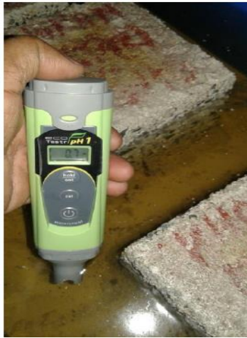
Fig 3.19. pH test of Sulphuric acid used for experiment.
