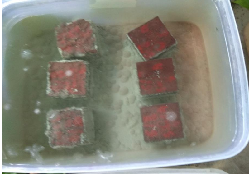
Fig 4.66 Sample exposed to Sulphuric Acid of 4% Concentration
