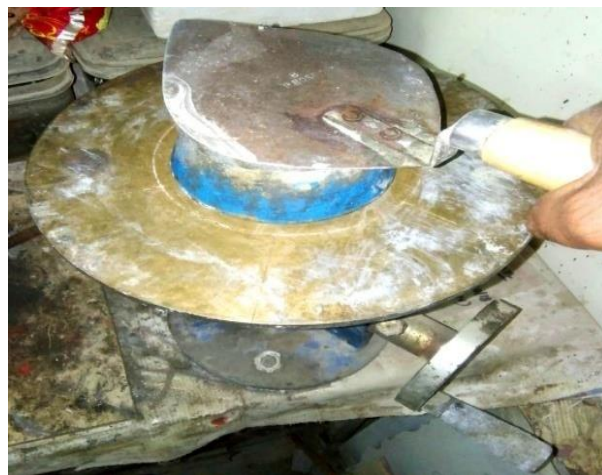
Fig 4.1 Flow table test setup
