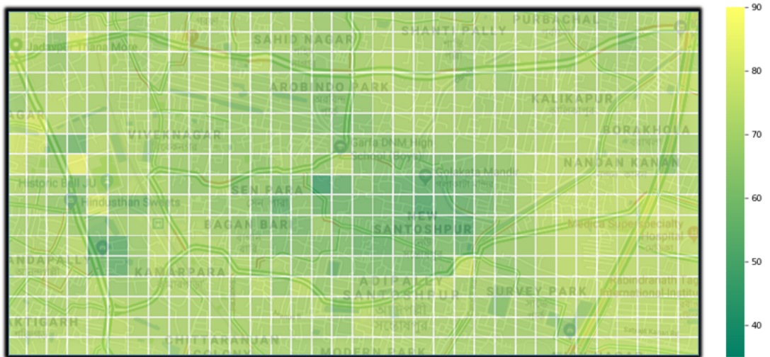
FIGURE 5.7: Noise pollution map generated by I-Grid-MSM method in final iteration.
