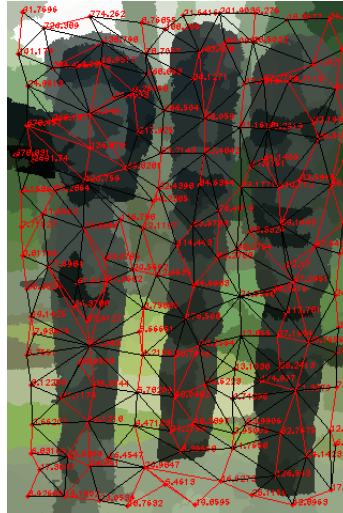
FIGURE 3.6: The neighboring graph showing the edges between nodes. Where Red colored edge denotes that two superpixels should be merged and Black edge denotes two superpixel cannot be merged
