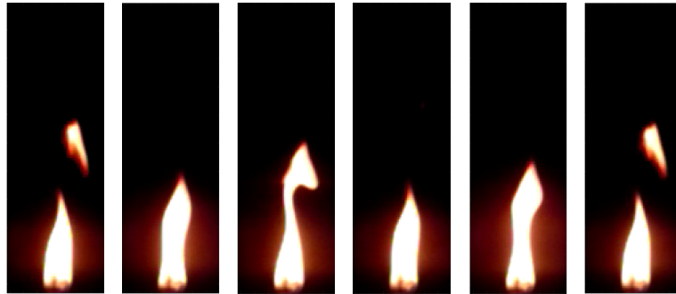
Figure 4.4: Flame images of a solitary candle flame oscillator (CFO) comprising five candles. The snapshots are captured at an interval of 0.0375 seconds.
