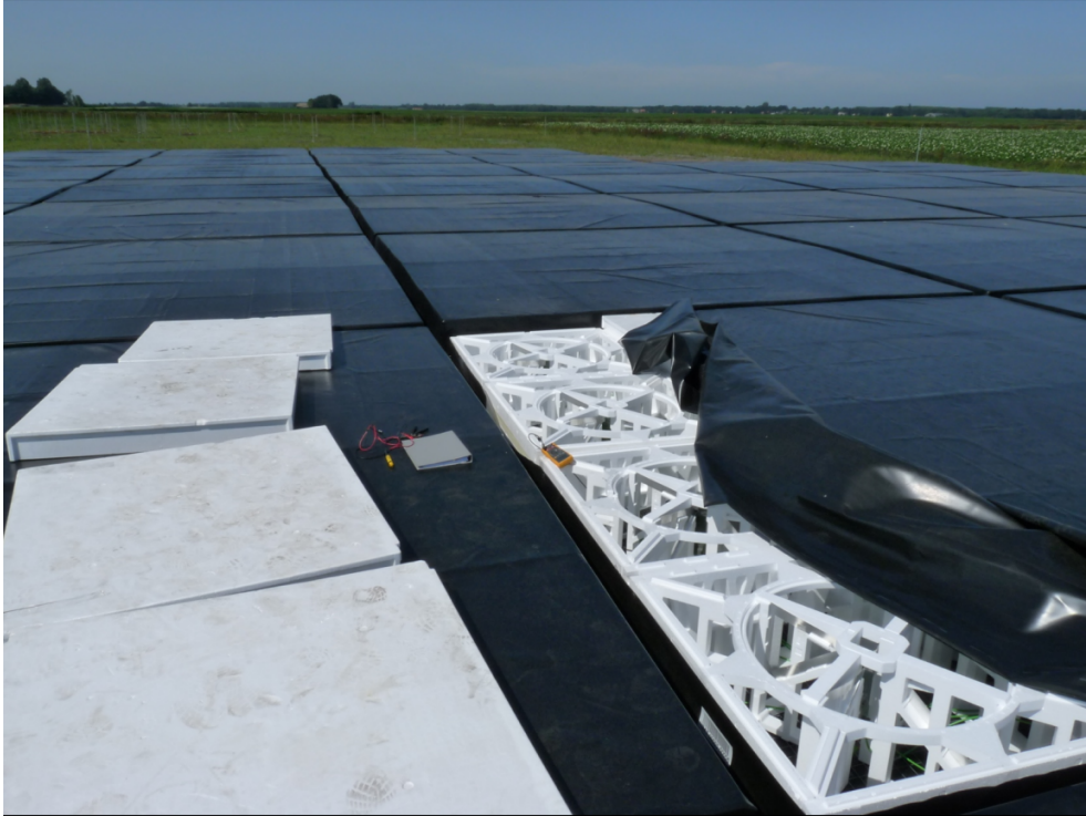
Figure 2.5: A single LOFAR HBA tile in close-up. The real dipole assembly has been partially revealed by removing the protective cover. It is possible to see the circular dipole rotation process. This image is taken from van et al.(2013).
