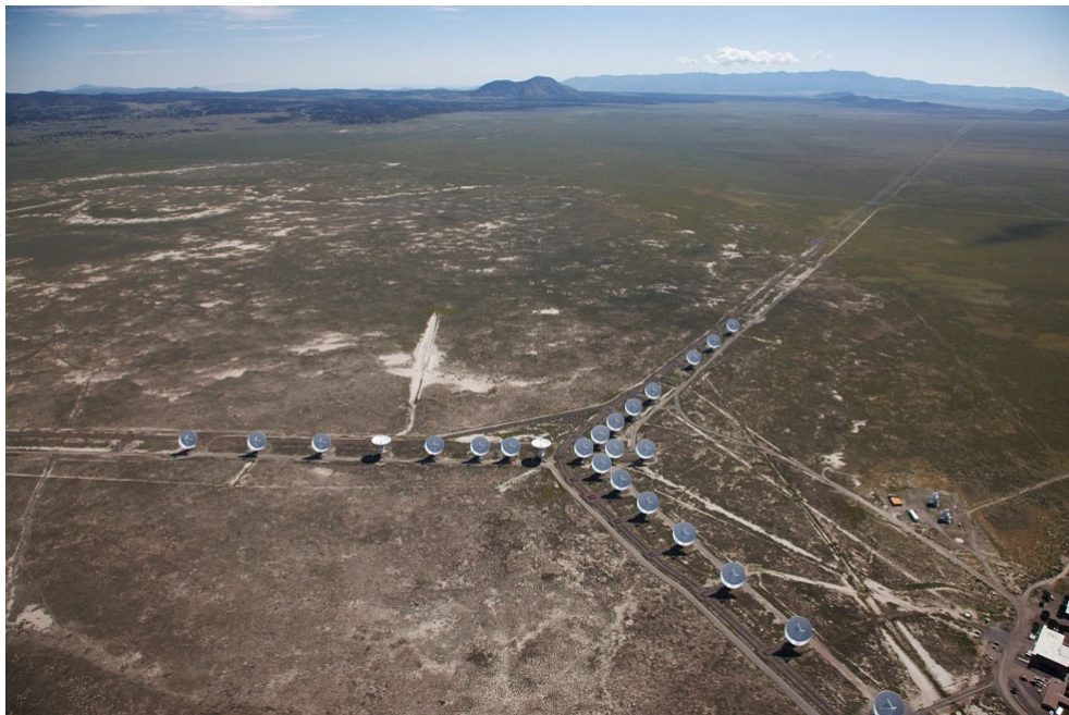
Figure 2.2: This image shows the 'Y'-shape array of VLA. Each array contains nine telescopes.
