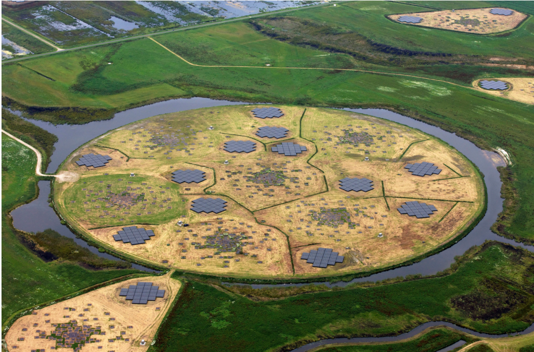
Figure 2.3: An aerial image of the Superterp, the LOFAR core's heart centre, taken in August 2011. The six core stations that make up the Superterp are all contained within the big circular island. In the top right and lower left corners of the picture, three more LOFAR core stations can be seen. These core stations each include two substations with 24 high-band antenna tiles each and a field of 96 low-band antennas. This image is taken from van et al.(2013).
