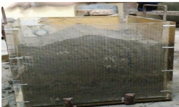
Fig. 4.15 Site elevation of Earthen Dam
