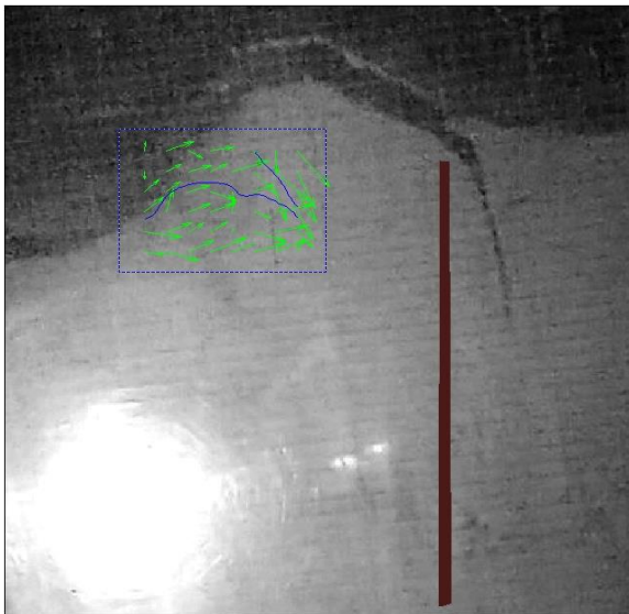
Figure 4.47(a): Flownet under rise up condition for 20 m long sheet pile at 2B/8 from downstream end, time=1 hour
